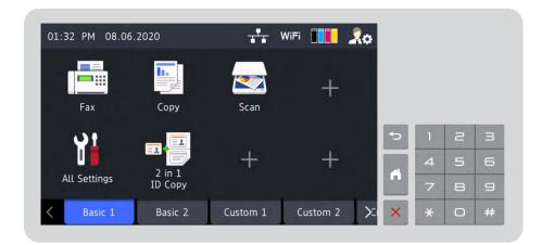
Remote Panel offers remote access to the front panel of the device through an Embedded Web Server (EWS). Enables remote configuration, as well as checking machine status, error conditions, and service reports. Helps reduce personal contact with the printer.
